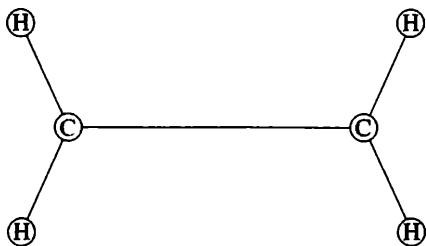
Figure 7.4 The planar structure of the ethylene molecule, C_2H_4 .
