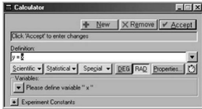
CI Figure 7.3 The calculator window. This small version of the calculator window opens when the Calculate button is pressed. The calculator will be used to enter formulas that handle the values measured by the sensor. The computer will perform the calculations automatically as the sensor takes data. (Reprinted courtesy of PASCO Scientific.)
