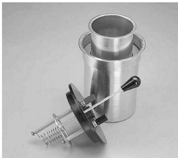
Figure 24.1 Joule heat determination. (a) The circuit diagram for the experimental procedure to measure joule heat. See text for description. (b) An electric calorimeter. (Photo Courtesy of Sargent-Welch.)
