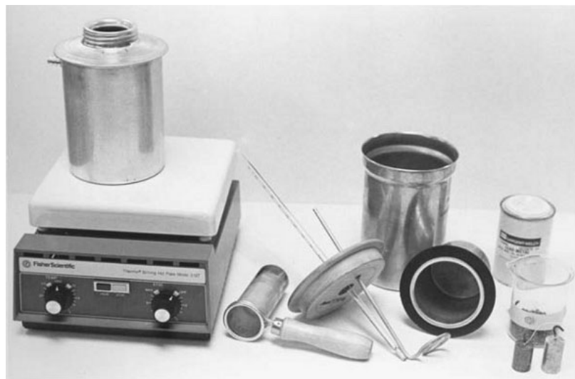
Figure 17.1 Apparatus for measurement of specific heats. Metal shot or a piece of metal (right) is heated with boiling water in the container on the hot plate. The metal is then placed in a known amount of water in the calorimeter, which insulates the system from losing heat. The inner calorimeter cup is shown with its dark, insulating ring lying in front of the outer cup. A thermometer and stirrer extend through the calorimeter cover. (Cengage Learning.)
