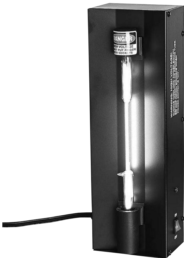
Figure 31.3 Experimental apparatus. A gas discharge tube and power supply. (Photo Courtesy of Sargent-Welch.)
