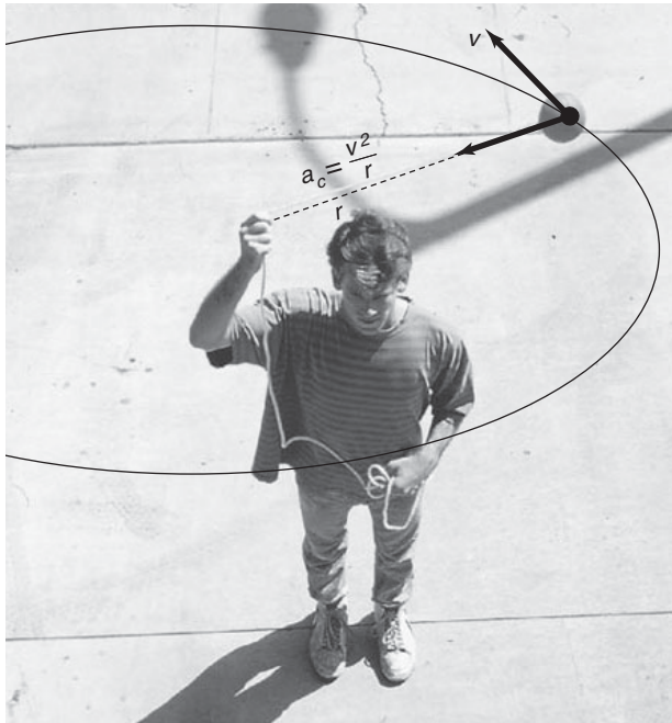
Figure 9.1 Centripetal acceleration. An object in uniform circular motion must have a centripetal acceleration with a magnitude of a_c = v^2/r directed toward the center of the circular path. In the case of swinging a ball on a rope around one’s head, the centripetal force F_c = ma_c is supplied by the person and transmitted through the rope. (Tony Freeman/PhotoEdit.)
