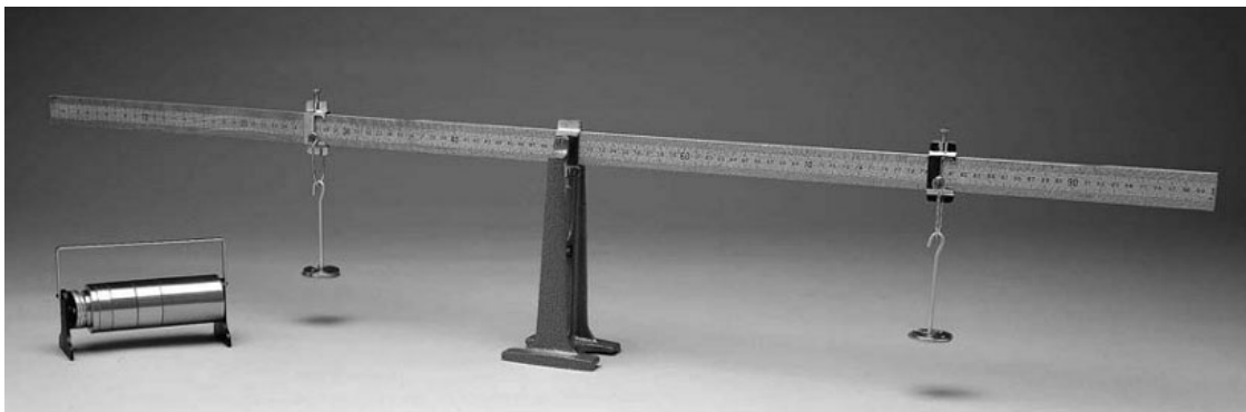
Figure 12.4 Torque apparatus. Example of experimental setup and equilibrium conditions. (Photo Courtesy of Sargent-Welch.)
