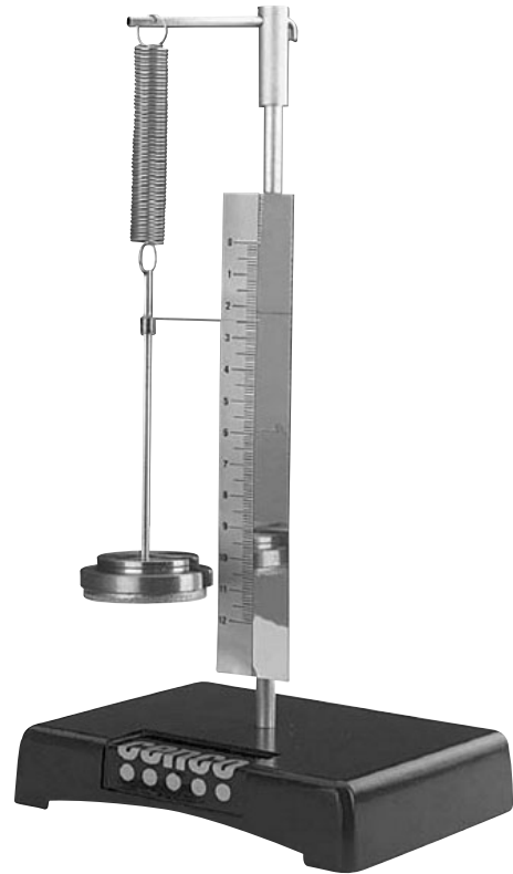
TI Figure 14.3 Hooke's law apparatus. The variables of Hooke's law ( F = mg and x ) are measured using spring elongation. (Photo Courtesy of Sargent-Welch.)
