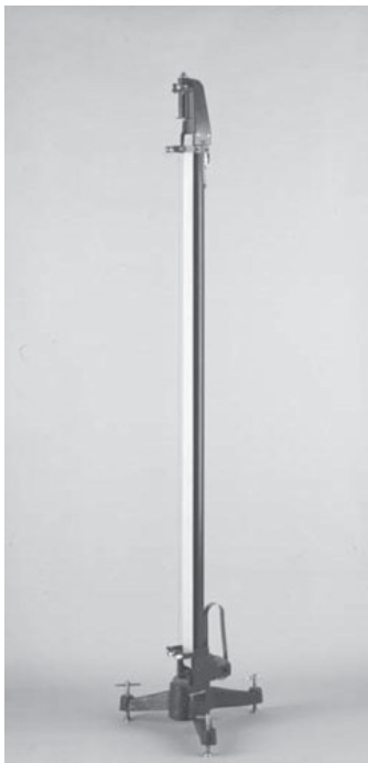
TI Figure 4.1A Spark timers. Types of free-fall spark timer apparatuses. (Photos (left and center) Photo Courtesy of Sargent-Welch. (right) Harvard)
