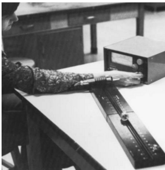
Figure 33.2 Apparatus for radioactive experiments. The standard side-window Geiger tube probe on the mounting board is connected to a count-rate meter. A radioactive source is on the board in the foreground. Notice the radioactivity warning sign on the source. (Cengage Learning.)
