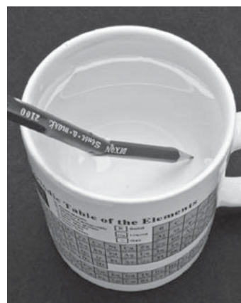
Figure 27.1 Refraction. Because of refraction the pencil appears to be bent. (Charles D. Winters/Cengage Learning.)
