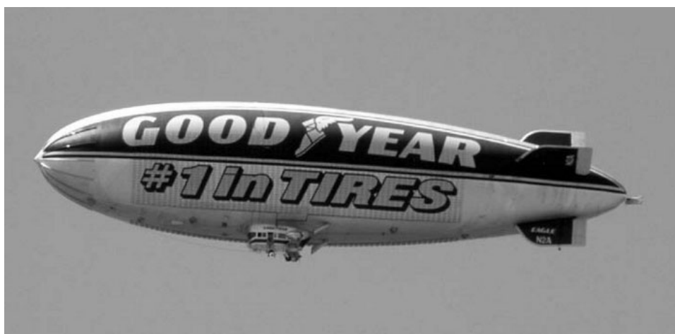
Figure 18.1 Gas buoyancy. Archimedes' principle applies to fluids—liquids or gases. Here, a helium-filled blimp floats in air. (Bill Aron/PhotoEdit.)
