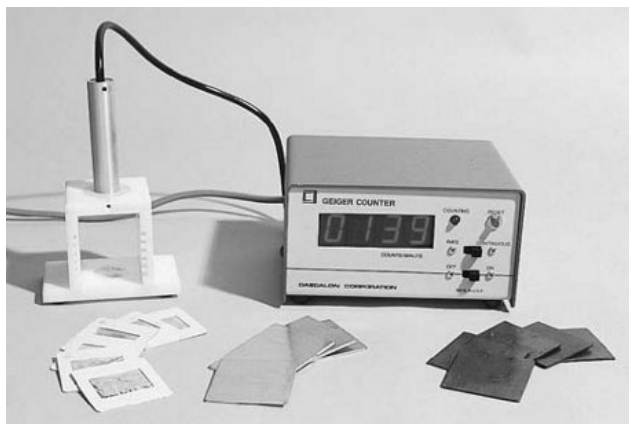
Figure 35.3 Geiger counter setup. (Fisher Scientific Company, LLC.)
