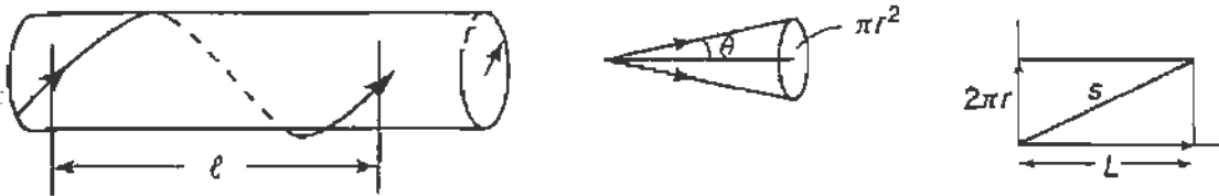
FIGURE 5.27 Layout of the fiber winding on a cylinder. Here the fiber length is s and the radius of the cylinder r .
