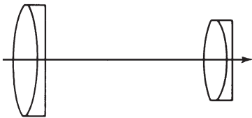
Figure 13.23 The Petzval portrait lens.
